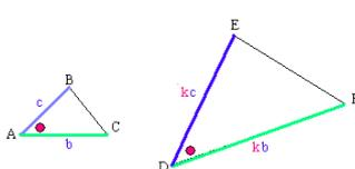
$$\begin{aligned} \otimes \quad |\hat{A}| &= |\hat{D}| \\ \otimes \quad \frac{|AB|}{|DE|} &= \frac{|AC|}{|DF|} = k \end{aligned}$$
